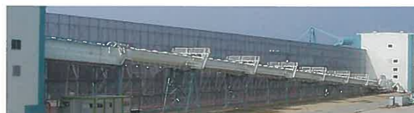
5,000t/h エア浮上コンベヤ (Uパイプ式) 5,000t/h Air Floating Conveyor (U-pipe type)
