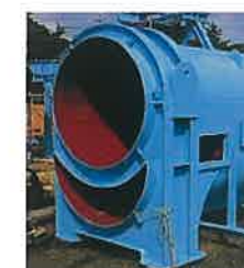
5,000t/h エア浮上コンベヤ (Uパイプ式) 5,000t/h Air Floating Conveyor (U-pipe type)
