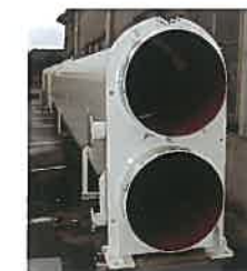
5,000t/h エア浮上コンベヤ (Uパイプ式) 5,000t/h Air Floating Conveyor (U-pipe type)
