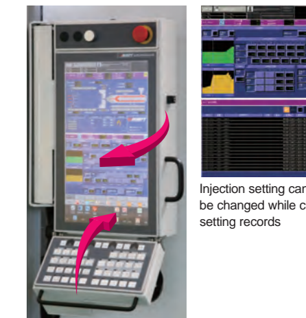
Control panel with two independent screens Swing and tilt function
